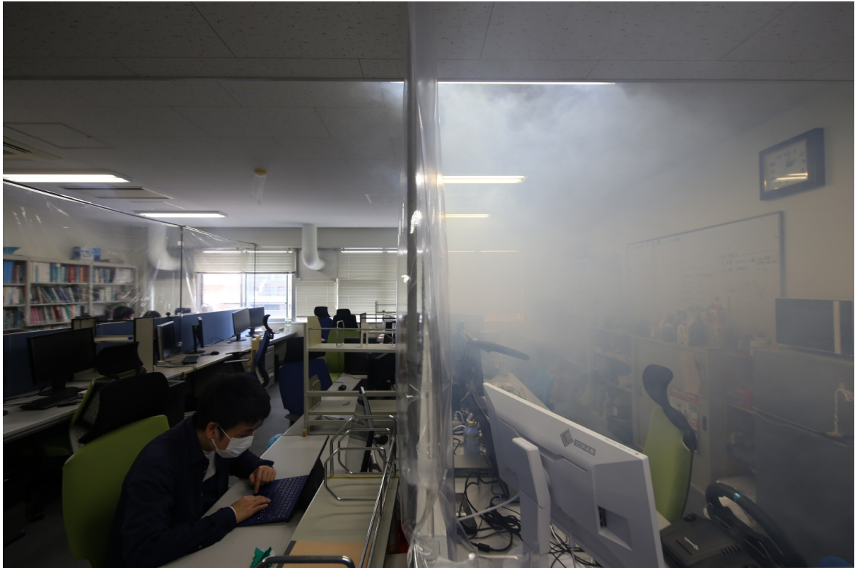
Experimental recreation of an office that faced COVID-19 outbreaks. The plastic sheeting drastically reduces airflow across compartments and traps microdroplets within a compartment. Photo courtesy: Yo Ishigaki of the University of Electro-communications, Japan.
